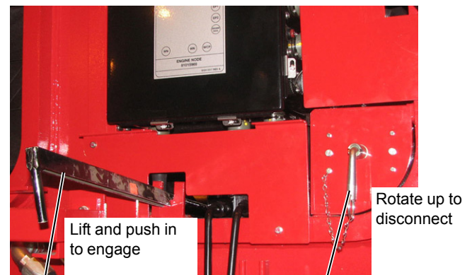
Right Side of Crane Clutch Lever Shown in Engaged Position Battery Disconnect Switch Shown in Connected (Closed) Position
