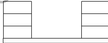
99,500 lb Crane Counterweight 6 side boxes
