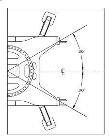
Operating Restrictions on Jacks and One Crawler Down (two jacks with one crawler on ground)
