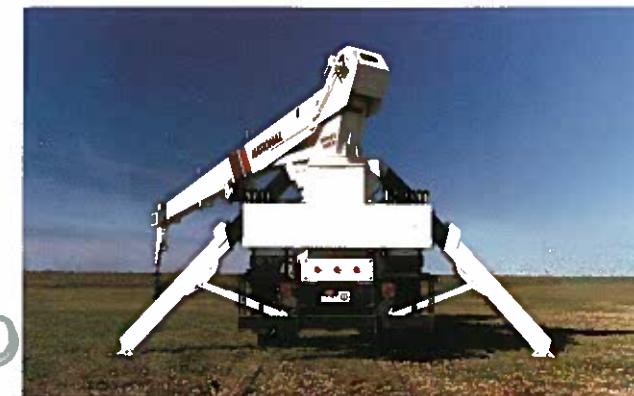
Rear view demonstrates the wide 18' stance of the mainframe outriggers. These quickly stow within 96" for fast take-down for transport.
