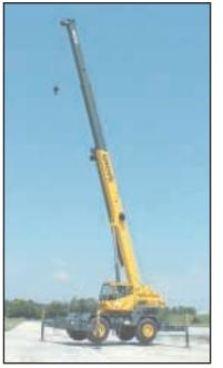
31 - 75 ft. (9.4 -22.9 m) three section full power boom; maximum tip height: 84 ft. (25.6 m)
