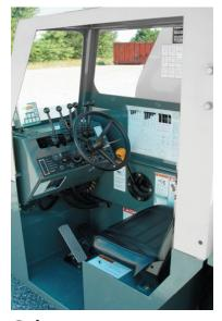
**Cab Standard:** Open air cab shell with overhead safety glass. **Optional:** Closed cab with split hinged door, heater/defroster, and all window glass.
