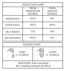
1) The rated loads are the maximum lifting capacities as determined by operating radius only. Any combination of boom lengths and angles may be used to obtain operating radius. The operating radius is the horizontal distance from a projection of the axis of rotation to the supporting surface, before loading, to the center of vertical hoist line or tackle with load applied.
