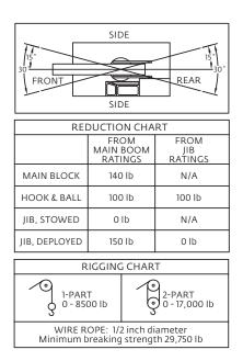
1) The rated loads are the maximum lifting capacities as determined by operating radius only. Any combination of boom lengths and angles may be used to obtain operating radius. The operating radius is the horizontal distance from a projection of the axis of rotation to the supporting surface, before loading, to the center of vertical hoist line or tackle with load applied.
