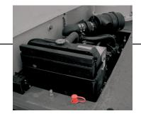
**Engine (Tier IV) Standard:** Cummins QSB 3.3 L turbo-charged diesel rated at 74,5 kW (100 bhp) at 2600 rpm.
