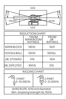
The rated loads are the maximum lifting capacities as determined by operating radius, boom extension and boom angle. The operating radius is the horizontal distance from a projection of the axis of rotation to the supporting surface, before loading to the center of vertical hoist line or tackle with load applied.
