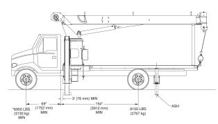
Configuration 3 with Torsion Box – 180° Full Capacity Work Area
