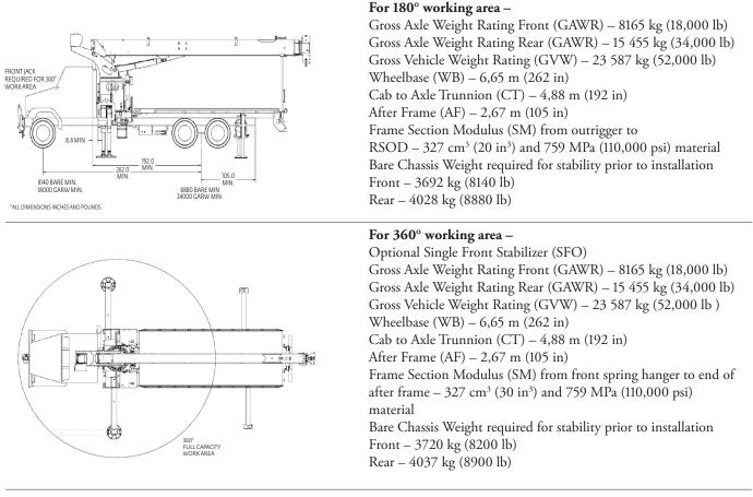
Note: Chassis will require extended front frame rails for SFO addition.
