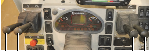
Remote Control Valves (in operator cab)
