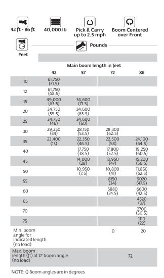
Lifting capacities at zero degree boom angle
