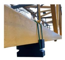
The elastic band holds the wedge in place during mast handling. The height of the wedge guarantees sufficient space to prevent hand injuries.
