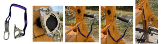
This lockable system prevents the risk of pins falling when the crane is dismantled. - Anti-vibration tool to remove pins diameter 40 and 60 mm
