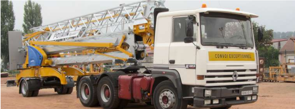
Transport crane fully ballasted
