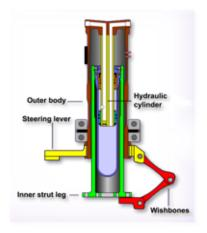
The MegaTrak Suspension strut comprises a hydraulic cylinder for the suspension function. The hydraulic cylinder rotates in the outer body of the strut to give the steering function.
