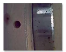
Unprotected cylinder rods will develop corrosion in the underlying steel, breaking through the chrome surface. Ultimately the chrome surface is destroyed, damaging the cylinder seals, leading to leakage and failure of the cylinder.
