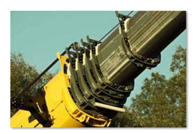
Smooth boom operation on a telescopic crane is a fundamental requirement to all lifting duties. Owing to the construction of modern pinned booms with relatively thin steel sections and large wear pads, this has never been more important. An appropriate lubricant with special properties is required.
