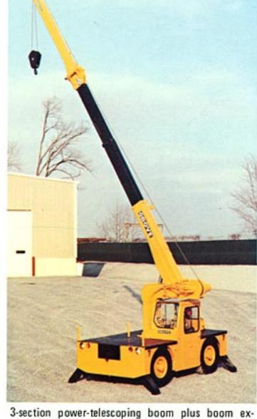
3-section power-telescoping boom plus boom extension provides a tip height of 32 ft. 6 in. (9.9m) and a horizontal reach of 27.6 ft. (8.4m). Notice the excellent visibility provided by the large windows and skylight. Carry-deck area is 45 sq. ft. (42m<sup>2</sup>).
