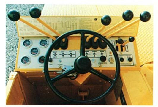
The arrangement of controls is consistent in all Grove cranes. Notice the neat, business-like appearance and convenience of crane function controls to driving controls.
