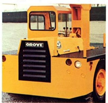
Serviceability is always an important consideration. On the Model 24, the engine position provides ready access to routine service needs.
