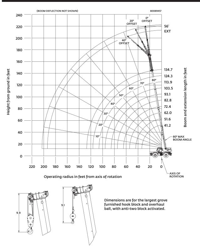
Working range diagram with bi-fold extension and insert
