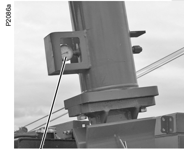
Hydraulic Pressure Gauge at Base of Both Mast Stops
