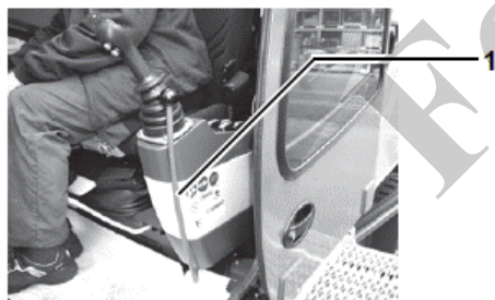
Fig. 9: Safety lever activated (pulled back)
