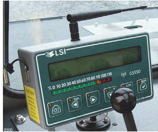
Load Indicator / Rated Capacity Limiter Indicator Panel
