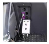
• Use the upper connector for RCL, the lower connector for ECOS
