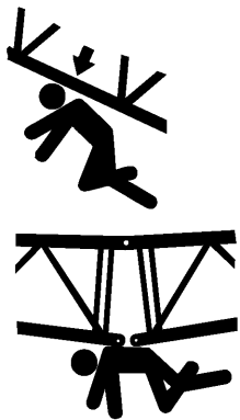
Falling Boom Hazards (Crush Hazard)
