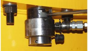
To use this material, please refer to the maintenance section of your crane manual which defines precisely the general rules for tightening your slewing ring bolts.
