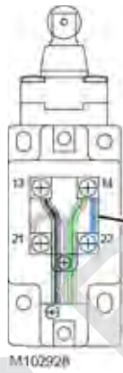
Limit Switch Wiring
