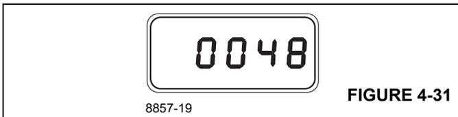
Set the desired remaining heating period with the buttons (6), (Figure 4-21) and (7) in the flashing display. You can set a remaining time of 1 to 120 minutes.
