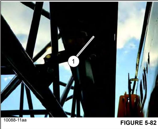
9. Make sure the attachment pin (1), (Figure 5-83) and retaining clip are in place that connects the ends of the fly section and the boom extension base section together.
