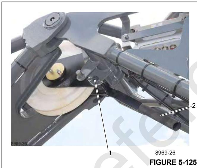
2. Hold the mast sheave by the handle (2), (Figure 5-125) and pull out the pin (1).
